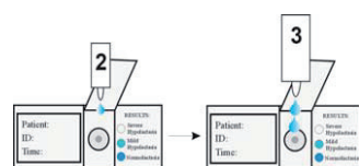
Figure2. Signal Reaction (glucose + color reagents -> blue color)
